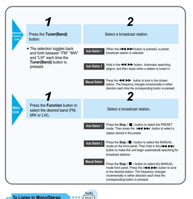
**Presetting stations** You can store up to: 15 FM stations • FM ..... Frequency Modulation • AM(MW) ..... Medium Wave 8 MW stations • LW ..... Long Wave 7 LW stations
